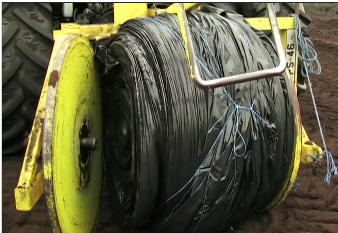
Plate 4-36 Polywrapper with the frame opened to allow access to the collected bale of polythene
